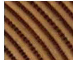
Berliner recording on lateral groove
